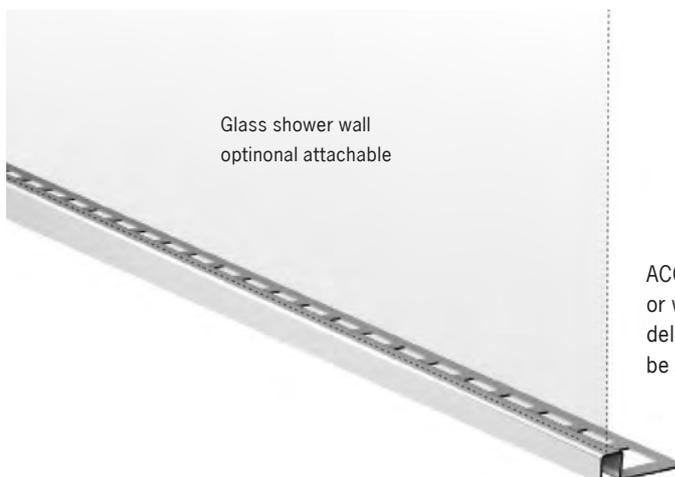
ACO ShowerStep has a 12 mm upper surface for use with or without glass shower wall. The width of the bar is chosen deliberately. Common shower partitions (up to 9 mm) can be used.
