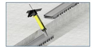
2. Apply the sealant on the of the connection area (male/female) and install the channels. Verify that the drainage line respects all the relative quotes.
